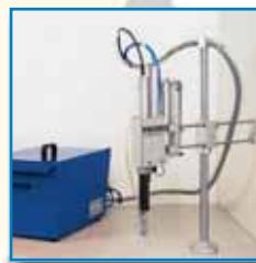
AUTOFEED HAND SCREWDRIVER WITH AUTOMATIC DOWN STROKE
