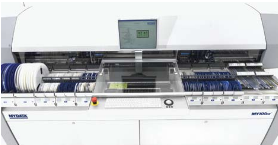
The MY100 offers up to 160 feeders in a compact footprint.
